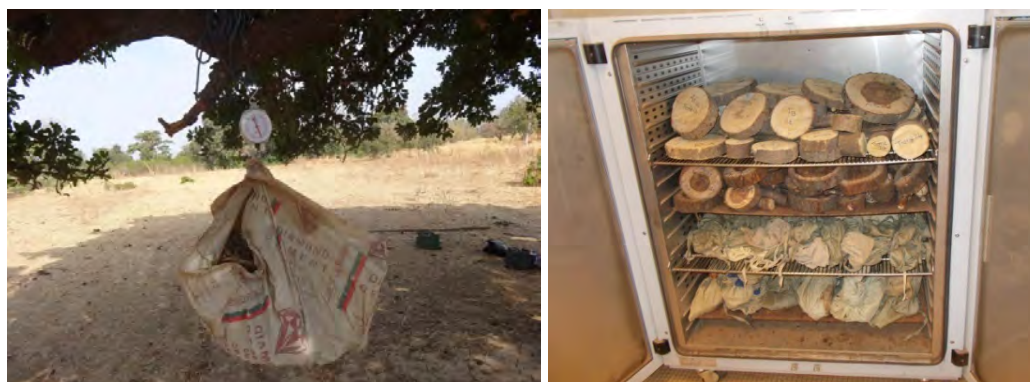
Figure 9. Sample weighing at field (left); Samples oven-drying (right).
