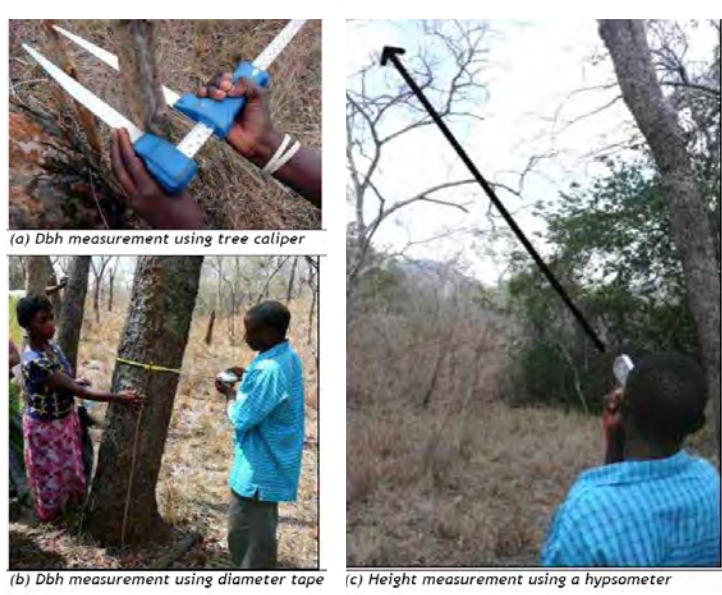
Figure 18. Measuring of tree parameters.
