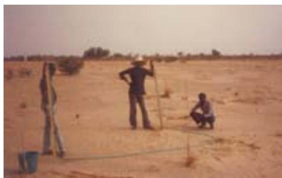
Water-tube level used to establish contour lines. /PDA/GIZ/Burkina Faso).
