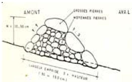
Permeable rock dike with filter layer.
