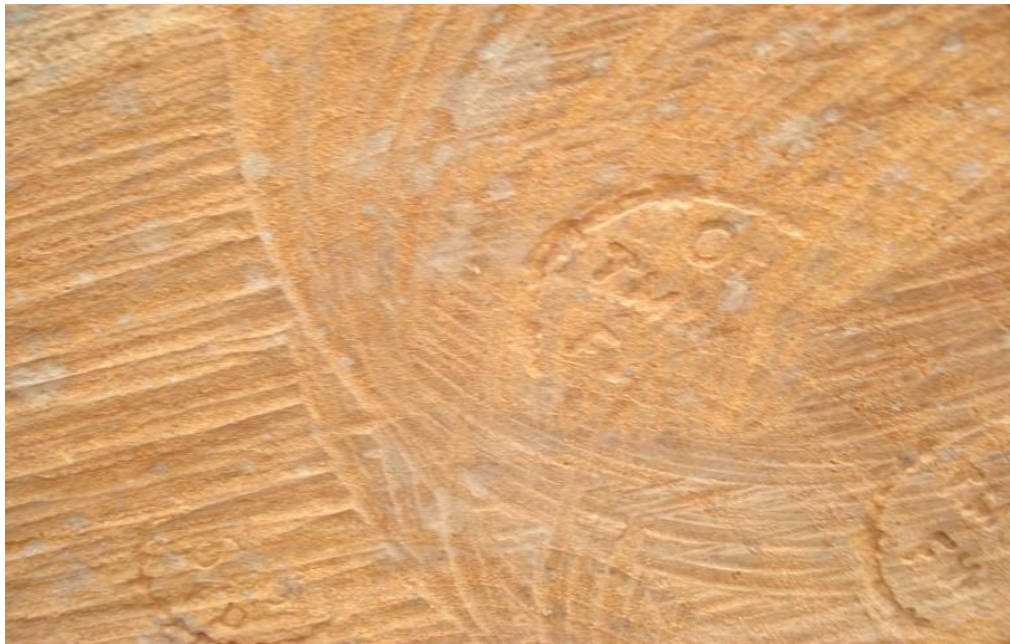
Plate 7: Timber regulation through pass hammering
