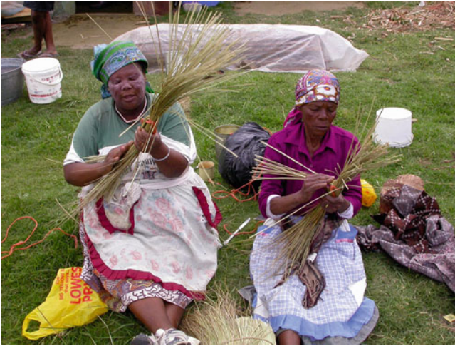
Fig. 5.3 Manufacturing grass brooms from Cymbopogon leaves in the Eastern Cape, South Africa (photo: Tony Dold)
